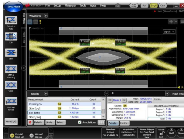
Figure 4a2 - T2 Output optical eye @LT
