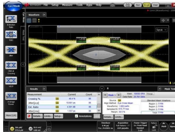
Figure 4a1 - T1 Output optical eye @LT
