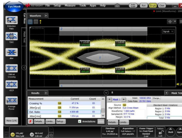
Figure 4b4 - T4 Output optical eye @NT
