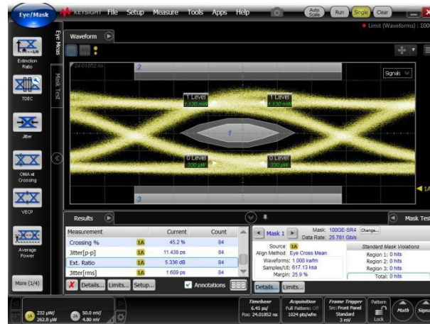
Figure 4c2 – T2 Output optical eye @HT
