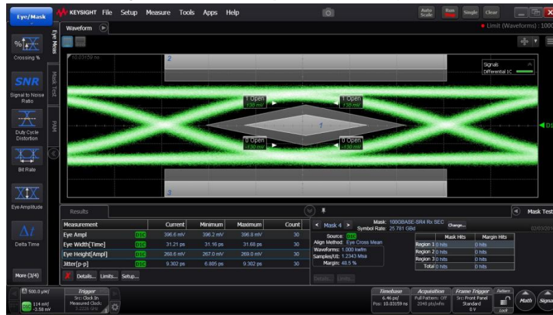
Figure 5b4 – R4 Output electrical eye @HT
