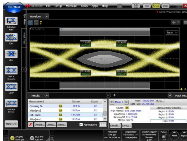
Figure 4a3 - T3 Output optical eye @LT
