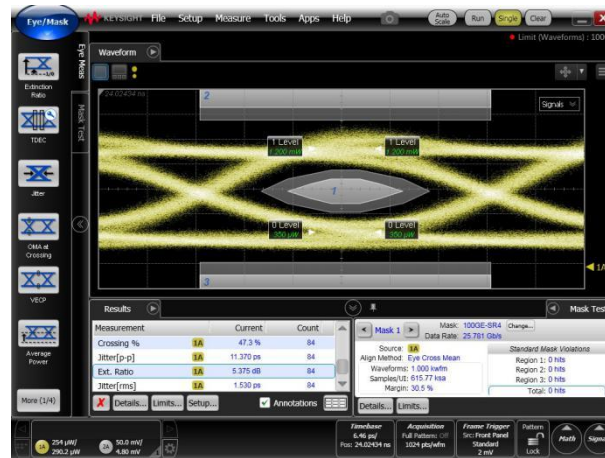
Figure 4c3 – T3 Output optical eye @HT
