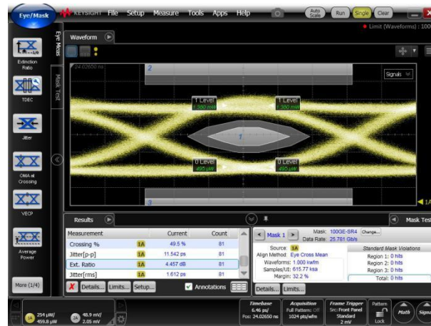
Figure 4b1 - T1 Output optical eye @NT
