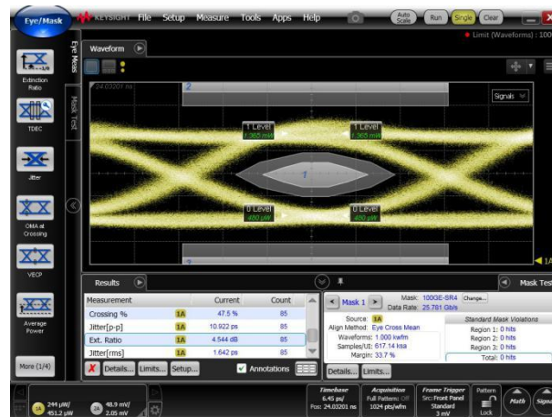
Figure 4b2 - T2 Output optical eye @NT
