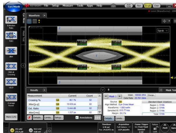
Figure 4c4 – T4 Output optical eye @HT
