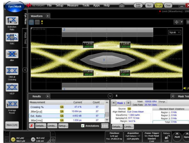
Figure 4b3 - T3 Output optical eye @NT
