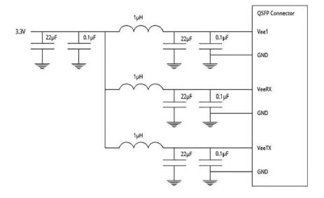
Figure 1. Host Board Power Supply Filtering
