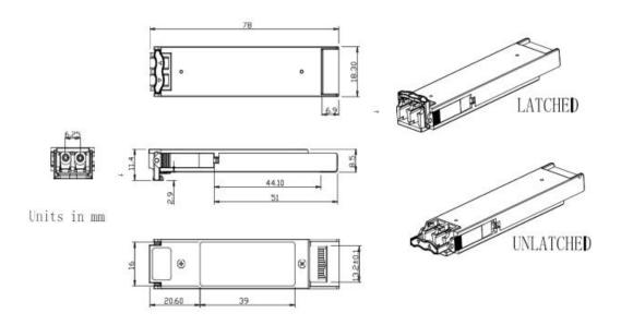
XFP Transceiver (dimensions are in mm)
