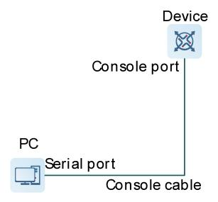
The first login to the device must be performed through the console port.
