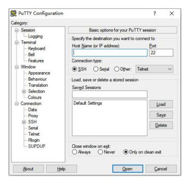
Click Serial in the left column. Set Speed (baud) to 115,200, Data bits to 8, Parity to None, Stop
