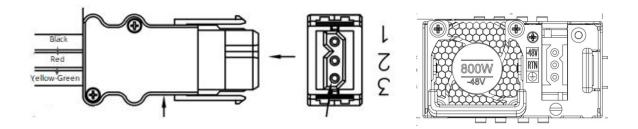
Figure 3-15 Installing the ND-PD800I-F
