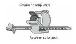
b. Thread the retainer strip through the hole at the bottom of the clamp and lock it into place, as shown in Figure 3-9. If you want to remove the strip, press the retainer strip latch and pull the strip out.
