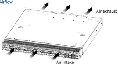
Figure 1-7 Rear-to-Front Airflow
