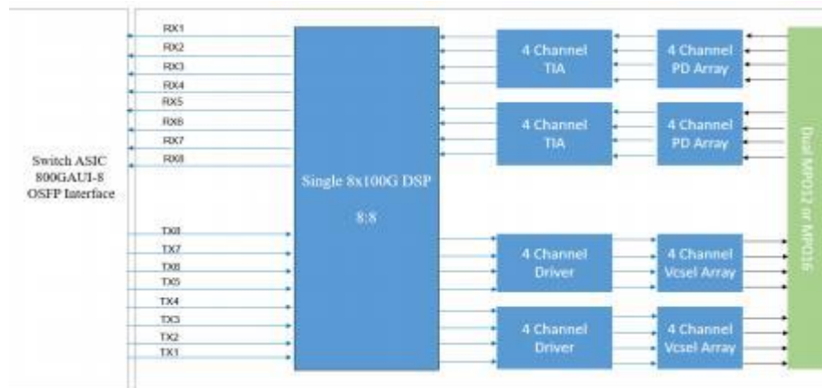
Figure 3. Transceiver Block Diagram
