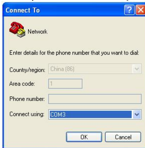
Figure 3-3 Set port connection
